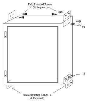
Figure 1 For best Flush Mounting results, recess face of enclosure's lip
